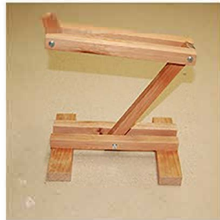
Drill a 4mm hole in the centre of two of the arms for the bottom of the frame. And 4mm holes, 11mm in from each end of the three remaining arms. Construct the lamp as illustrated here.
