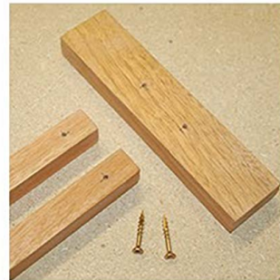
Secure the two 22 x 44 x 183mm feet to the bottom arms with the 25mm Eureka Cut Screws
